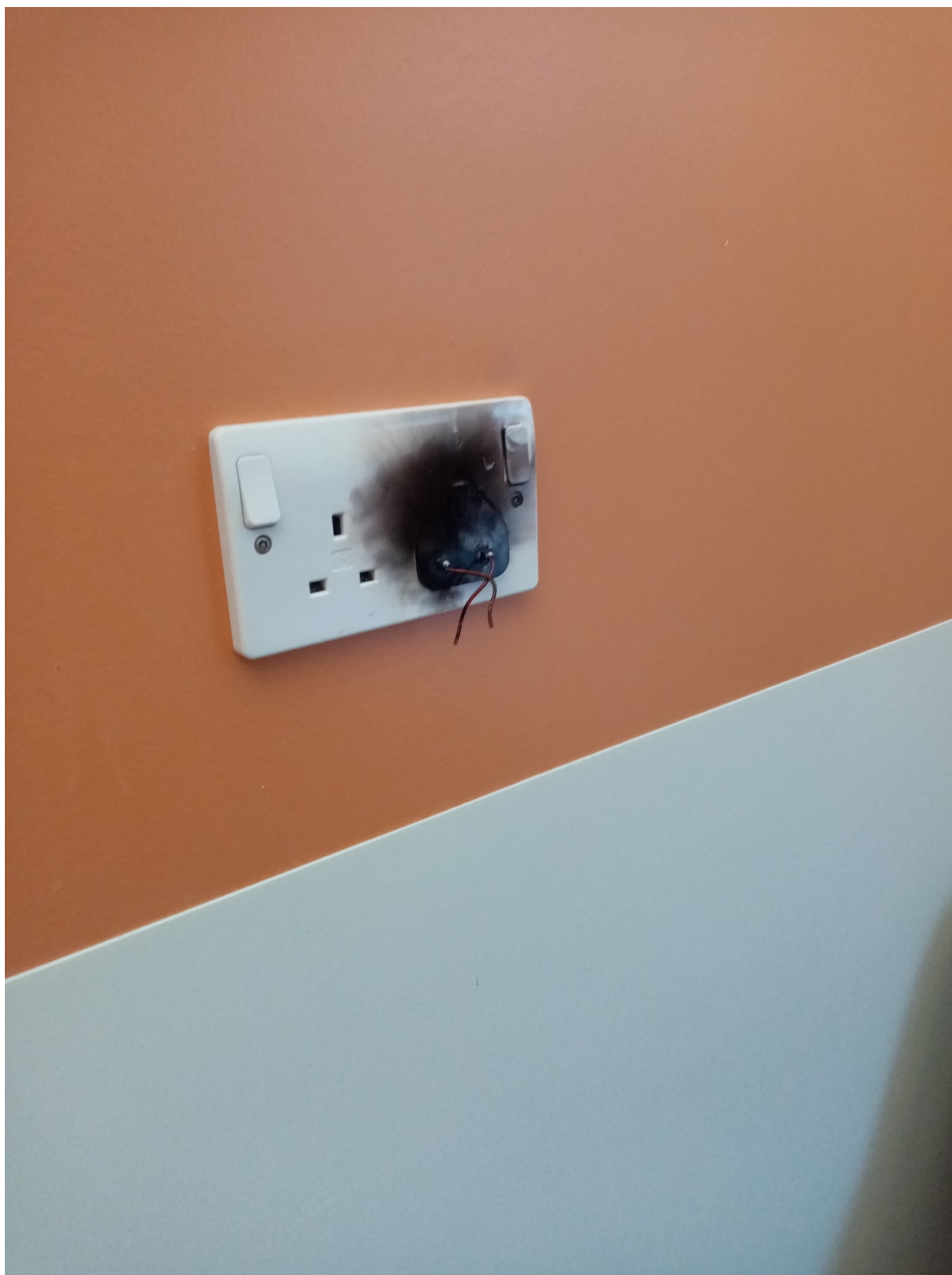
Image 1 – Scorched Wall Mounted Socket
